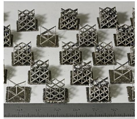
Metal parts made by additive manufacturing can be used in a number of industry applications as long as the material density meets that of traditionally-manufactured metal parts.
