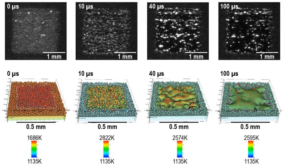
High-speed imaging of Seurat's process compared to simulation results indicated the simulation faithfully reproduced process timescales and physics.
