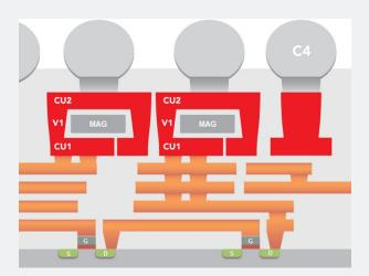
A cross-sectional view of a CMOS chip, Ferric's thin film magnetic inductor technology, shown in gray within the red box, is integrated into the back-end-of-line processing. *Illustration from Ferric, Inc.*
