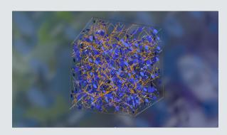
Lithium (gold) is added to aluminum (purple) to strengthen the resulting alloy. The model predicted alloy strength as a function of the percentage of lithium in the alloy. *Computational results image from LLNL*. LIFT partnered with Lawrence Livermore National Laboratory.
