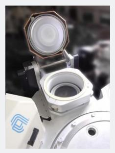
A single wafer process chamber used by Applied Materials to perform physical vapor deposition on any type of wafer, including the sapphire substrates used in this HPC project. *Photo from Applied Materials.*
