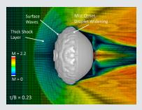
Vector plot colored by Mach number of a normal shock wave moving from left to right in air just having passed over a single droplet of water.
