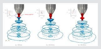
The interface between the fuel slurry and gas is shown at three different times. The primary jet is shown in red, and the atomized droplets are shown in blue. *Computational results images from Argonne National*
