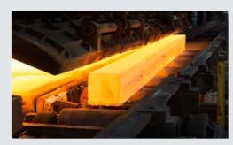
Semi-finished steel is reheated using a dynamically controlled process before entering the hot rolling operations. Reheating uses 70-80% of total energy used in rolling mills.
