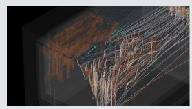
Visualization of molten glass flows generated by computer simulations. *Computational results image from LLNL*.
