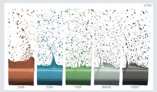
High-resolution peta-scale modeling of liquid atomization comparing different liquid rheologies. *Paint dispersion simulations from LBNL.*
