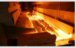
Raw materials entering a float-glass furnace tank for production of architectural glass. *Photo from Vitro Glass.*
