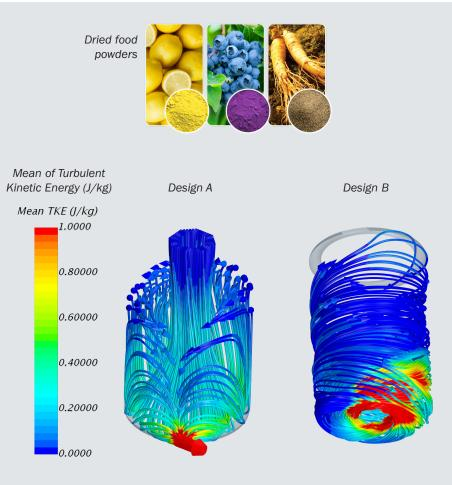
Two inlet design configurations were analyzed with a CFD model to improve the spray drying process. *Computational results images from Lawrence Livermore National Laboratory.*
