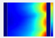
Cross sectional magnetic field of the magnetron in the high-power impulse magnetron sputtering system. *Computational* results image from LLNL.
