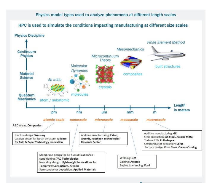
Ab Initio modeling framework rely on basic and established natural laws (first principles) in their calculations. These pico-scale models examine the parts of an atom, such as the position of the nucleus, photon flux, quantum efficiency, electron densities, energies, and other quantum chemistry phenomena. This level of analysis is used to better understand physical and chemical interactions that impact manufactured products. Factors modeled at this scale are ignored in larger scale models.
